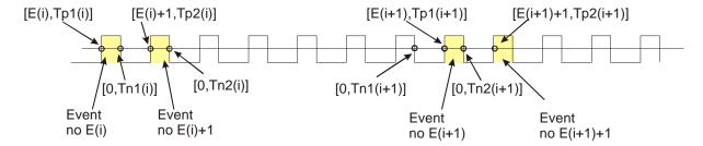
E(i) is the i:th sample of accumulated input cycles (ALL trigger events are counted and accumulated up to 160 MHz on input A or B,). E(i)=0 for the negative slopes, and the accumulated number of input cycles for the positive slope
