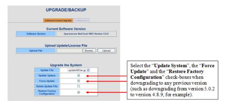
Reconfigure the settings as desired, or restore a previously saved config file from the version the software has just been downgraded to.
