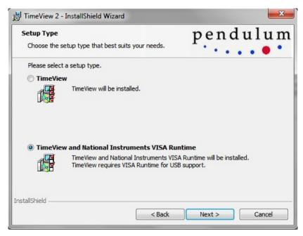
Please select TimeView and National Instruments Visa runtime. This will download USB drivers and allow the instrument to work in a National Instruments environment. Once the download and licensing issues are completed, measurements can be made. National Instruments Visa runtime is required even if you have USB drivers installed.
