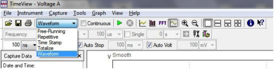
Going from **free-running** to **waveform** in **select capture type**, converts TimeView into an oscilloscope, displaying amplitude (volts) vs. time (ns).
