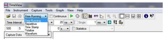
**Free running measurements:** Measures the variations of the measured parameter in real time. This mode also allows measurements of modulated signals (see below). Frequency range is up to 400 MHz (Ch A and B) and up to 3, 8, 16, or 20 GHz (Ch C). CNT-90XL has a range up to 60 GHz (This is the basic modulation domain capture mode setting).
