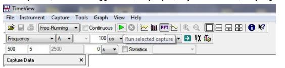
Press the **green** triangle on the front of TimeView to commence a measurement. The display will show a graph of frequency vs. time.
