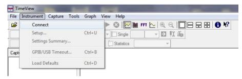
If the counter does not connect, then check the counter's interface setting in the "user option" menu on the counters front panel. Select "interface" and "type USB". After that, select "connect" again from TimeView.
