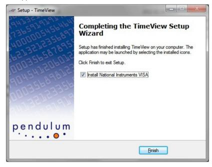
Please select Finish to install the National Instruments runtime. This will download USB drivers and allow the instrument to work in a National Instruments environment. Once the download and licensing issues are completed, measurements can be made. National Instruments Visa runtime is required even if you have USB drivers installed.
