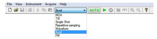
**MDA:** The purpose of this mode is to behave more like the Agilent 53310A Modulation Domain Analyzer, and to have settings that are familiar for oscilloscope users.
