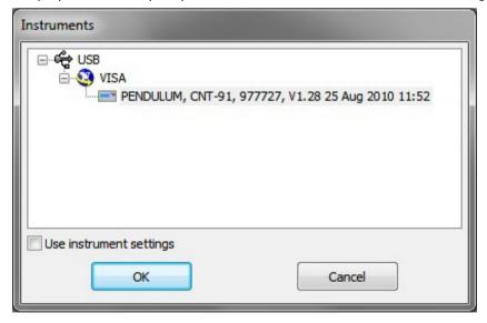
If the counter does not connect, then check the counter's interface setting in the "user option" menu on the counter's front panel. Select "interface" and "type USB". After that, select "connect" again from TimeView.
