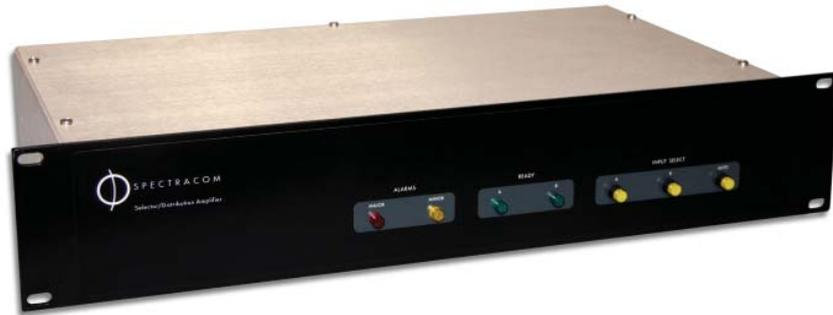
The Model 8143 Signal Selector/Distribution Amplifier detects failure of either input signal and provides manual or automatic switchover between two frequency sources. The selected input is distributed via 12 buffered output line drivers. In the automatic mode, Channel A is selected when it is present. Switchover occurs when Channel A is removed, when an alarm is sensed, or when a manual selection is made. In manual mode, switchover is operator-controlled.
