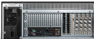
A CDM-5 is shown here synchronizing SDRs in a Skydel SDX GNSS Simulator System
