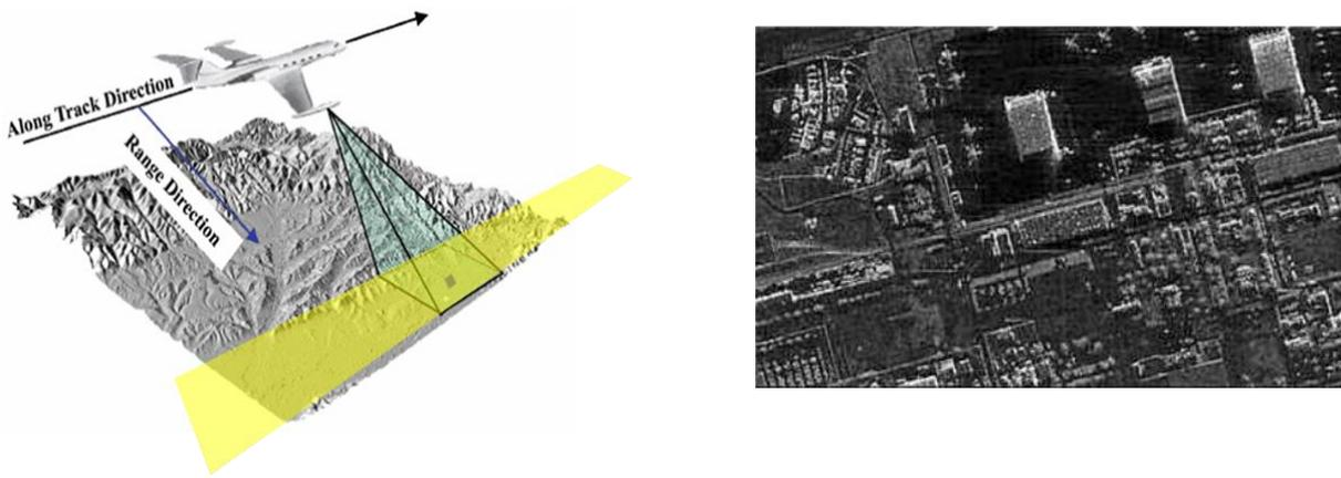
Fig 3: SAR imagery radar principle and SAR image
