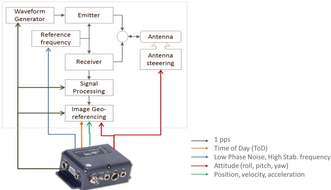
Fig 5: PNT requirements for a SAR radar subsystems
