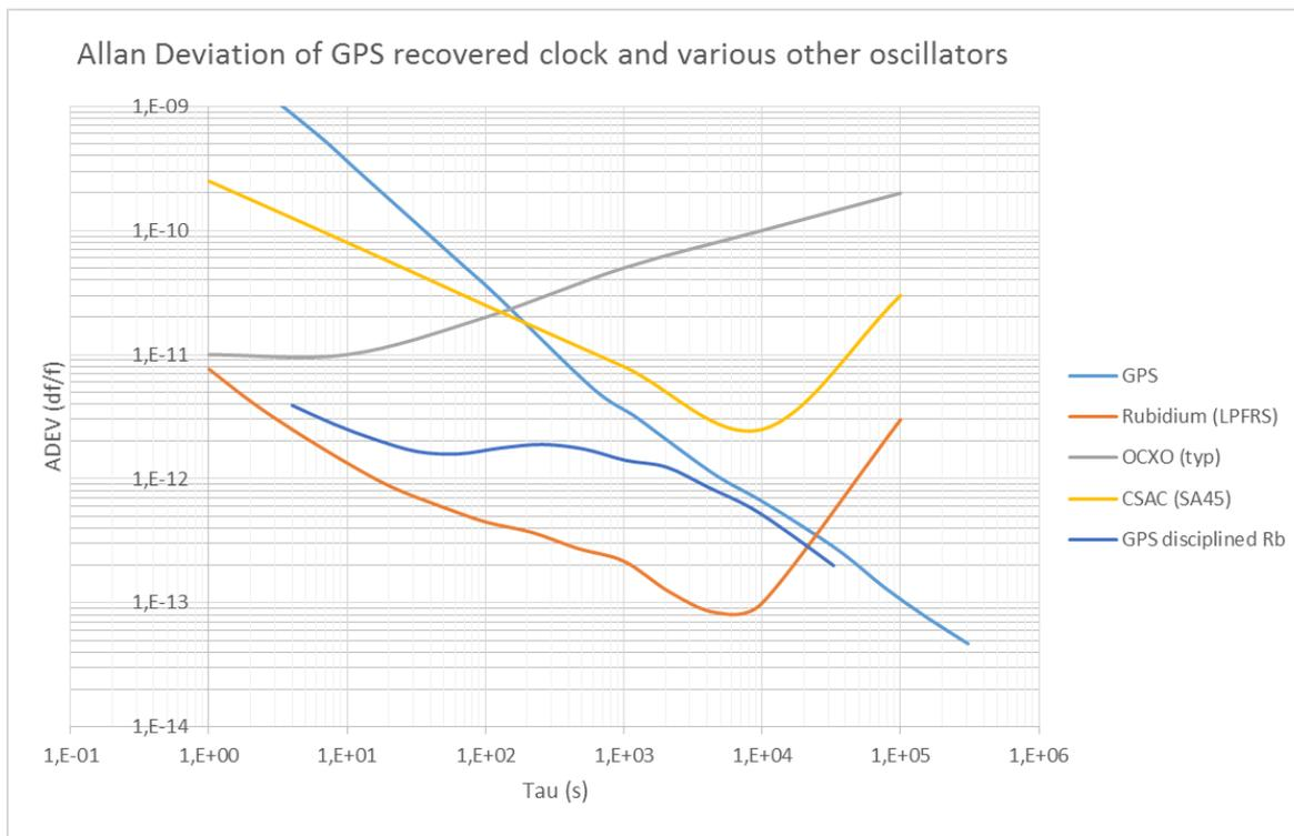
Fig 7: compared ADEV for GPS, and various types of oscillators
