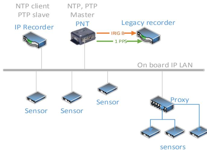
Fig 1: Typical timing architecture for an on-board timing system
