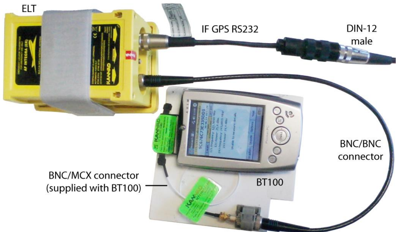
Figure 5: Example of BT100 Connection with ELT
