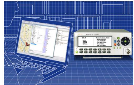
2. Connect the laptop to the simulator, edit the scenario as desired, and run the playback generator
