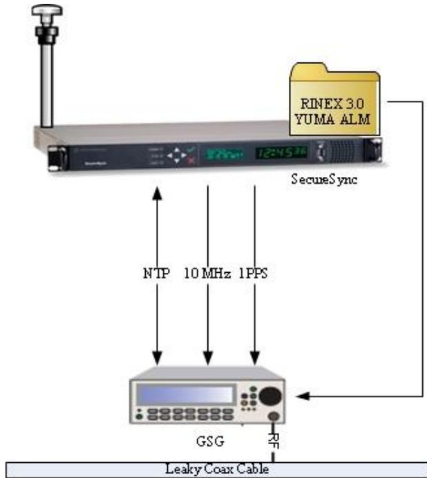
Fig. 1 Intelligent Repeater System – Single Zone
