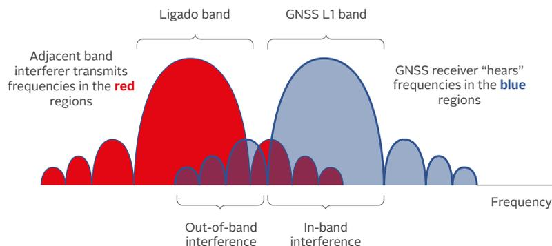
1. In-band interference – No transmitter is perfect. Some energy “spills” into the GNSS band from small bits of energy coming from the high-power transmitter. This can be reduced by better filtering at the transmitter.
