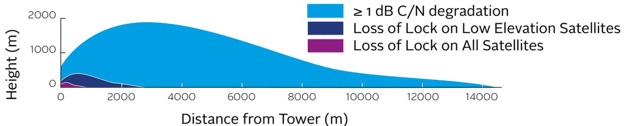
Figure ES-3: Impact of a 29 dBW Cellular Base Station Transmitting at 1530 MHz on a High Precision GPS/GNSS Receiver
