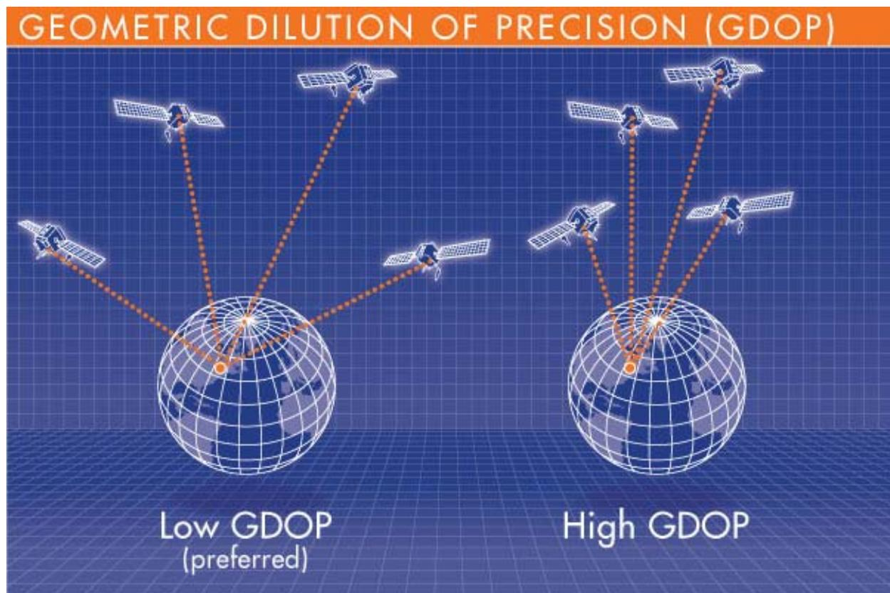
**Figure 1: A narrow spread of satellites results in a geometric dilution of precision**
