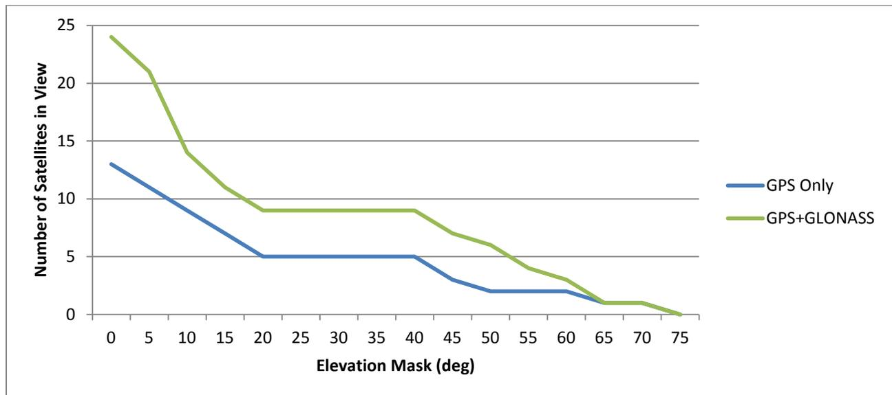
**Figure 3: When combining systems, a larger elevation mask can be tolerated**
