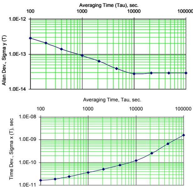
Figure 4. RAFS2 core model frequency and time stabilities
