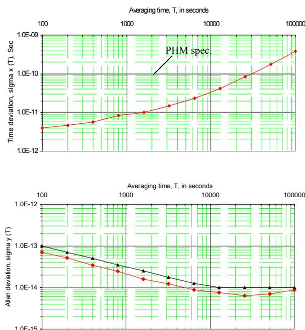
Figure 9. PHM EM frequency and time stabilities
