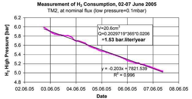
Figure 15. H2 consumption test
