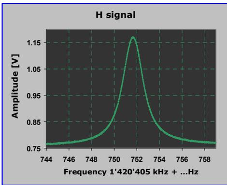
Figure 10. PHM atomic signal measured in FM1
