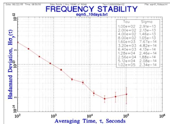
Figure 3. RAFS1 EQM frequency data and frequency stability
