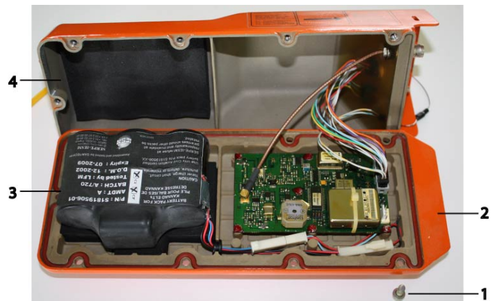
Figure 4: Opening / Closing the ELT (For P/N S1819502-02 Only)
