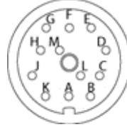
Figure 2: DIN-12 Connector Pin-out
