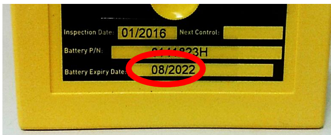
Battery expiry date on the ELT.
