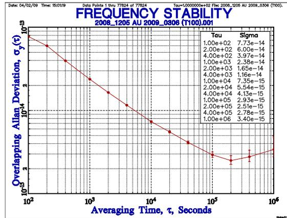
Figure 8. PHM QM1 frequency data and frequency stability (with drift)
