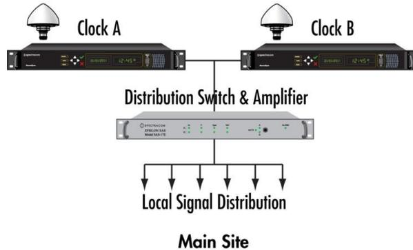
Figure A2: Local Distribution with Redundant Master Clocks
