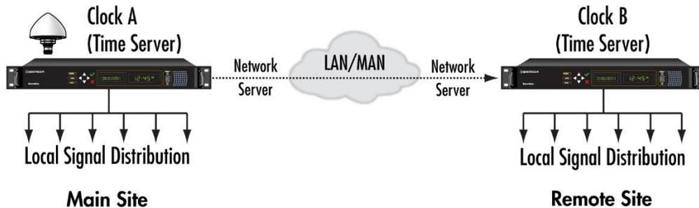
Figure C: Local Signal Distribution via Network Sync
