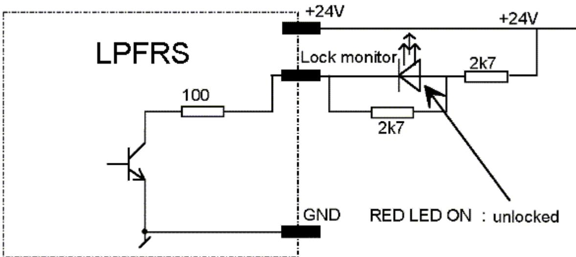
The lock monitor output can be directly connected to the CMOS load, or a pull-up resistor can be added for TTL compatibility.
