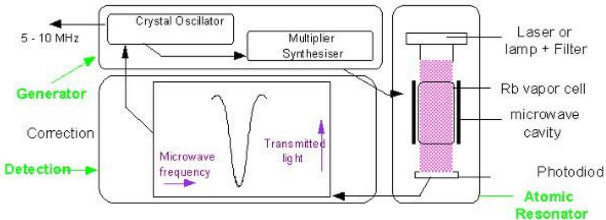
Fig. 2-2: Rubidium atomic clock principal block diagram
