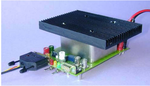
Fig. 2. First suggested mounting: the radiator is screwed to the RMO cover through 4 M3 screws. This solution is not suitable in a hermetic case, for the radiator is mounted horizontally.
