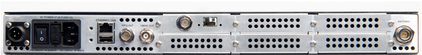
Base units include 10 MHz and 1PPS output signals, network port and choice of power, GPS reference, and internal oscillator options.
