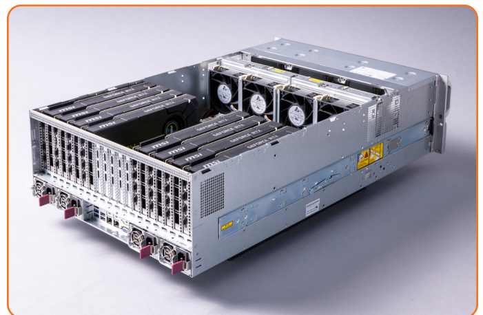
Pictured Above: Wavefront Node, generates IQ data per each element
