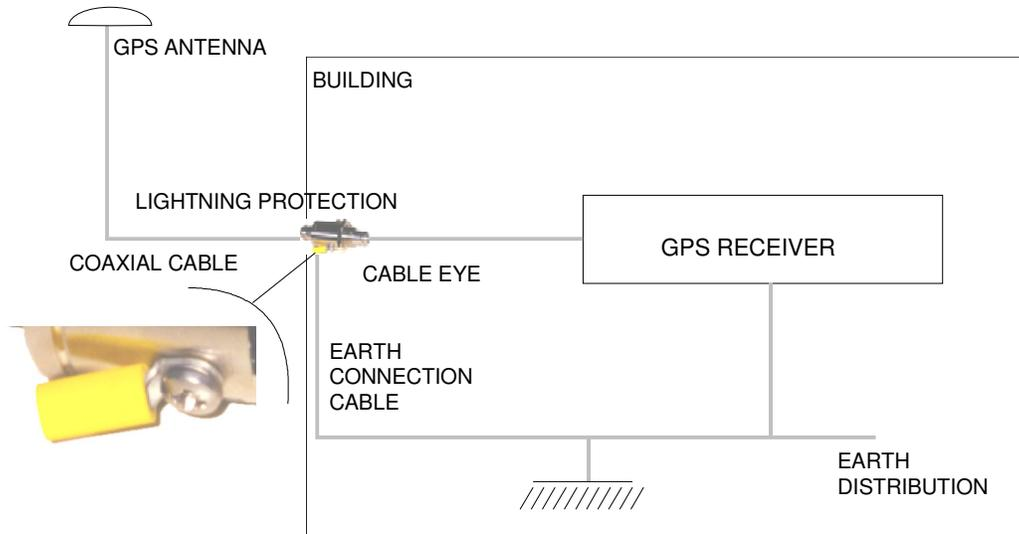
The lightning protection ground connection must have a very low impedance value. Use a section greater than 3mm<sup>2</sup> and the shortest possible length of cable between the protection and the building ground connection.
