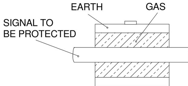
Once the energy from the lightning has been shunted to the ground, the gas returns to its initial state of rest as an insulator. GPS lightning protection, which is specifically designed for 1500 MHz, is totally user-transparent.
