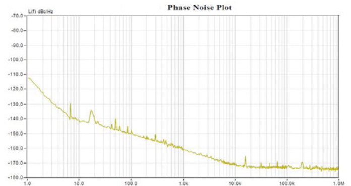
LNMO Phase noise at 10MHz
