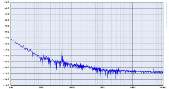
Typical MO LN Phase Noise at 10MHz
