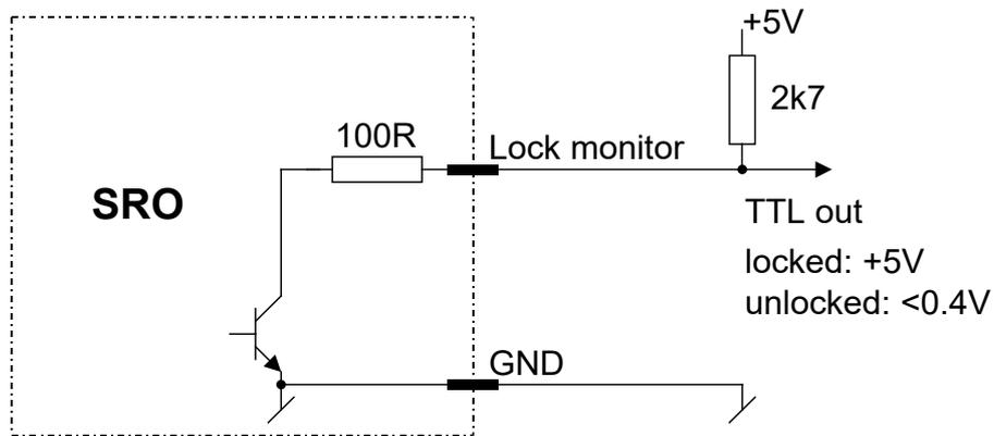
*Fig. 4-4: The lock monitor*
