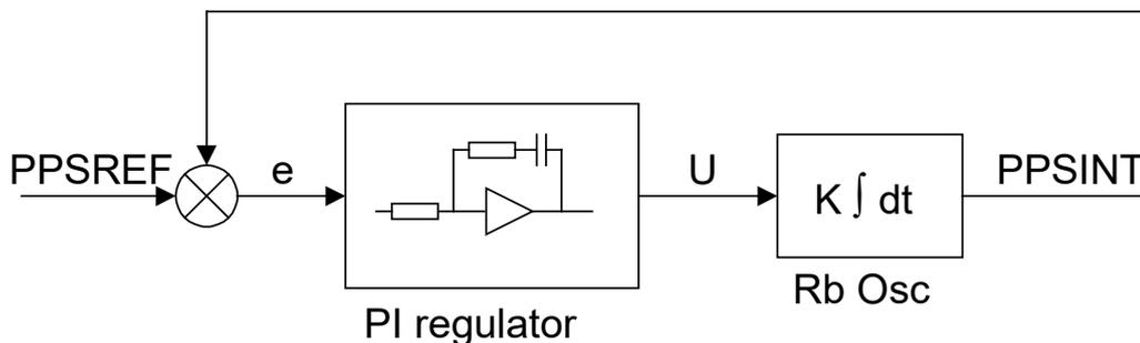
Figure 5 - Schematic of the PPSREF Regulation Loop
