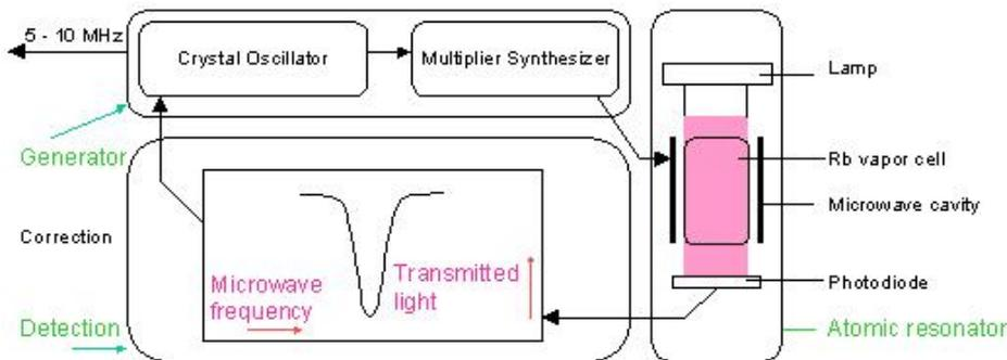
Figure 2 - Rubidium atomic clock block diagram.
