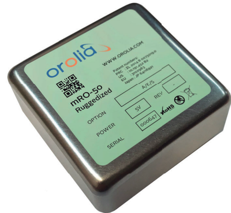
Miniature, Low SWaP-C, ultra-portable high precision & performance Atomic Frequency Source
