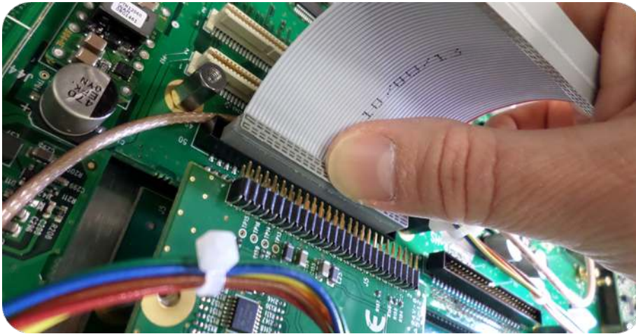
Figure 8: Ribbon cable installation
