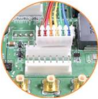
Figure 10: J19 Connector, seen from rear of unit.
