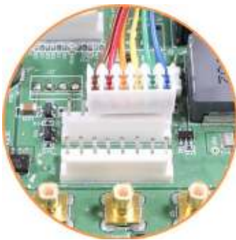
Figure 12: J19 Connector, seen from rear of unit.
