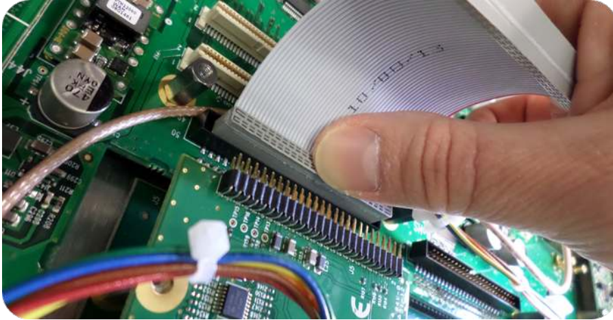
Figure 6: Ribbon cable installation
